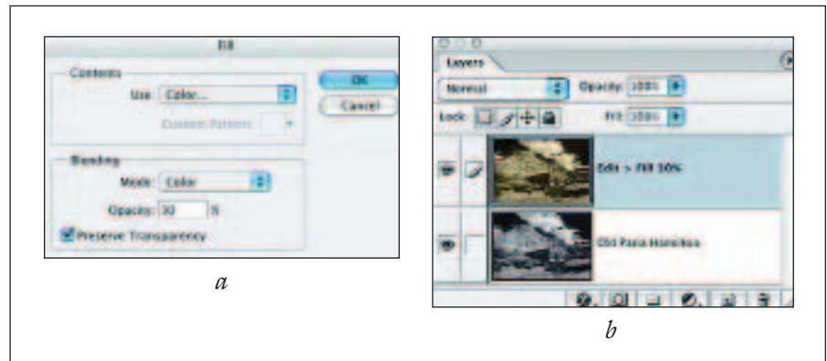
FIGURES 5-13A AND B. COLOR FILL. (a) The Fill dialog box, accessed from the menu item Edit>Fill. In addition to Color, options include Foreground Color, Background, Pattern, History, Black, 50% Gray, and White. (b) Layers palette after filling duplicate image layer with color.
